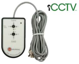
The inMotion inUTC-ZF is an optional iCCTV $^{\text{TM}}$  compliant product to enable advanced programming of inMotion cameras. The hand-held programmer is connected is via a simple Male / Female loop through BNC cable that is inserted in series with the video signal from the camera, to a monitor or control device. Once connected and activated, the programmer sends a telemetry signal back along the coax to enable and navigate around the On-Screen-Display menus of the connected inMotion camera.
